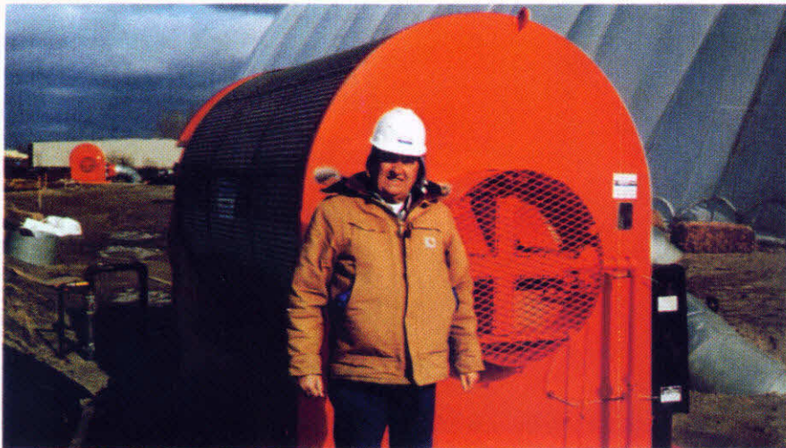
Thermal C/M Services' Mike Duke stands before one of two 4.5-million-BTU natural gas heaters supplied by BABFAR Equipment to inflate and warm the dome.
